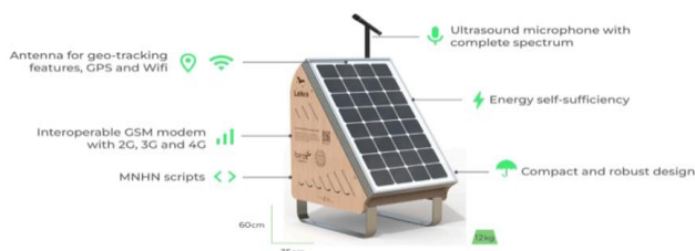
Figure 35. LEKO sensor description scheme (BIRDZ, 2025)
